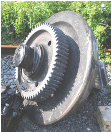
Right: Broken axle with bull gear
