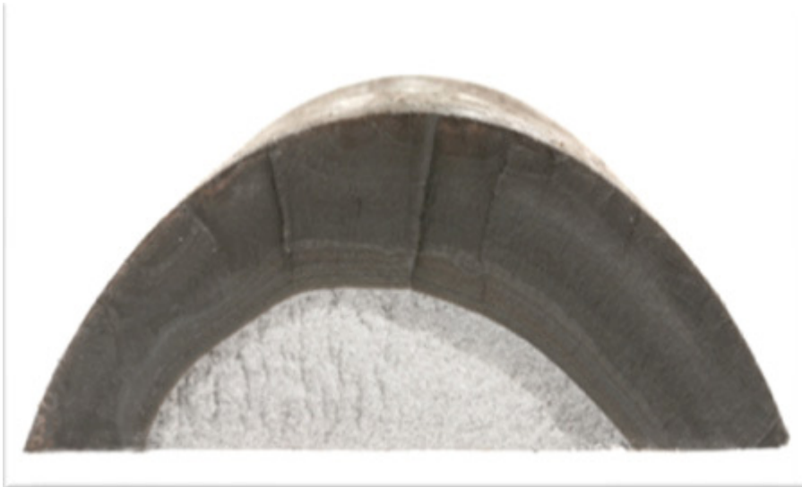
Photo 4. Close-up of secondary crack in axle No. 3
