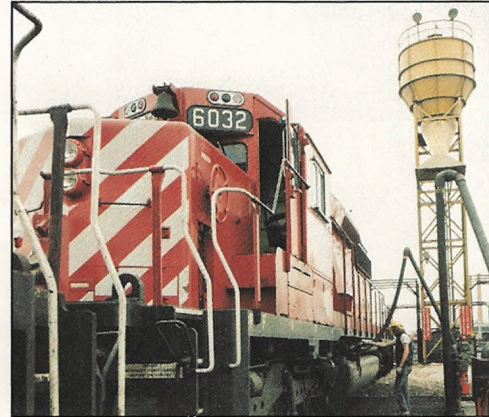
Fueling and sanding operations
