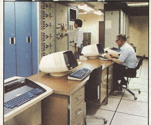
Above: From the Alyth control tower the train yard coordinator controls and monitors the entire humping operations and internal yard movements. Below: The retarder operator adds an extra measure of safety by being able to override potentially undesirable humping conditions.
