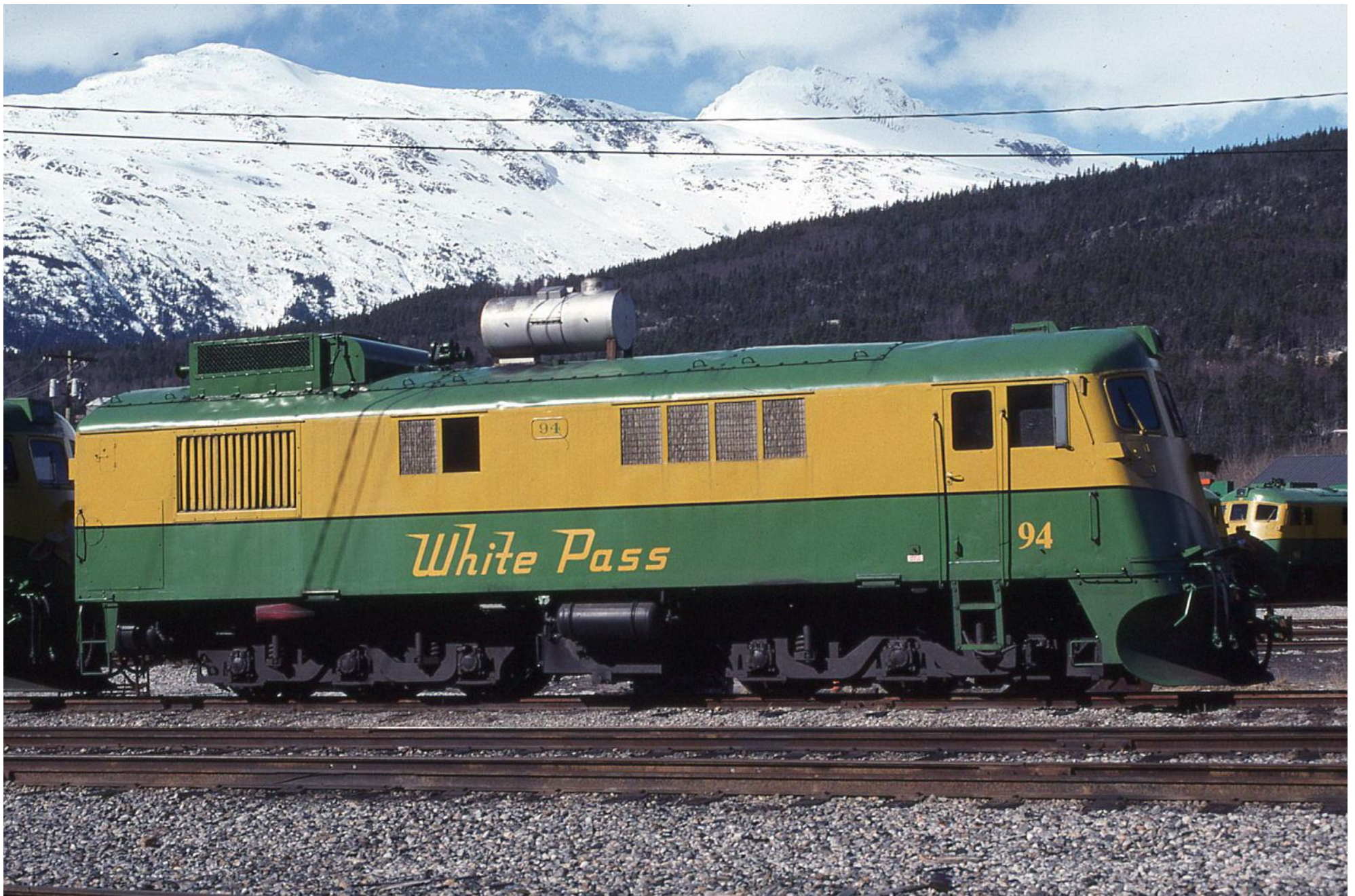
Unit #94 obtained a rather ungainly exhaust scrubbing device. Fortunately, the experiment was deemed a failure and the “tank” was removed. Skagway 4/6/01 Photo by Deane Motis
