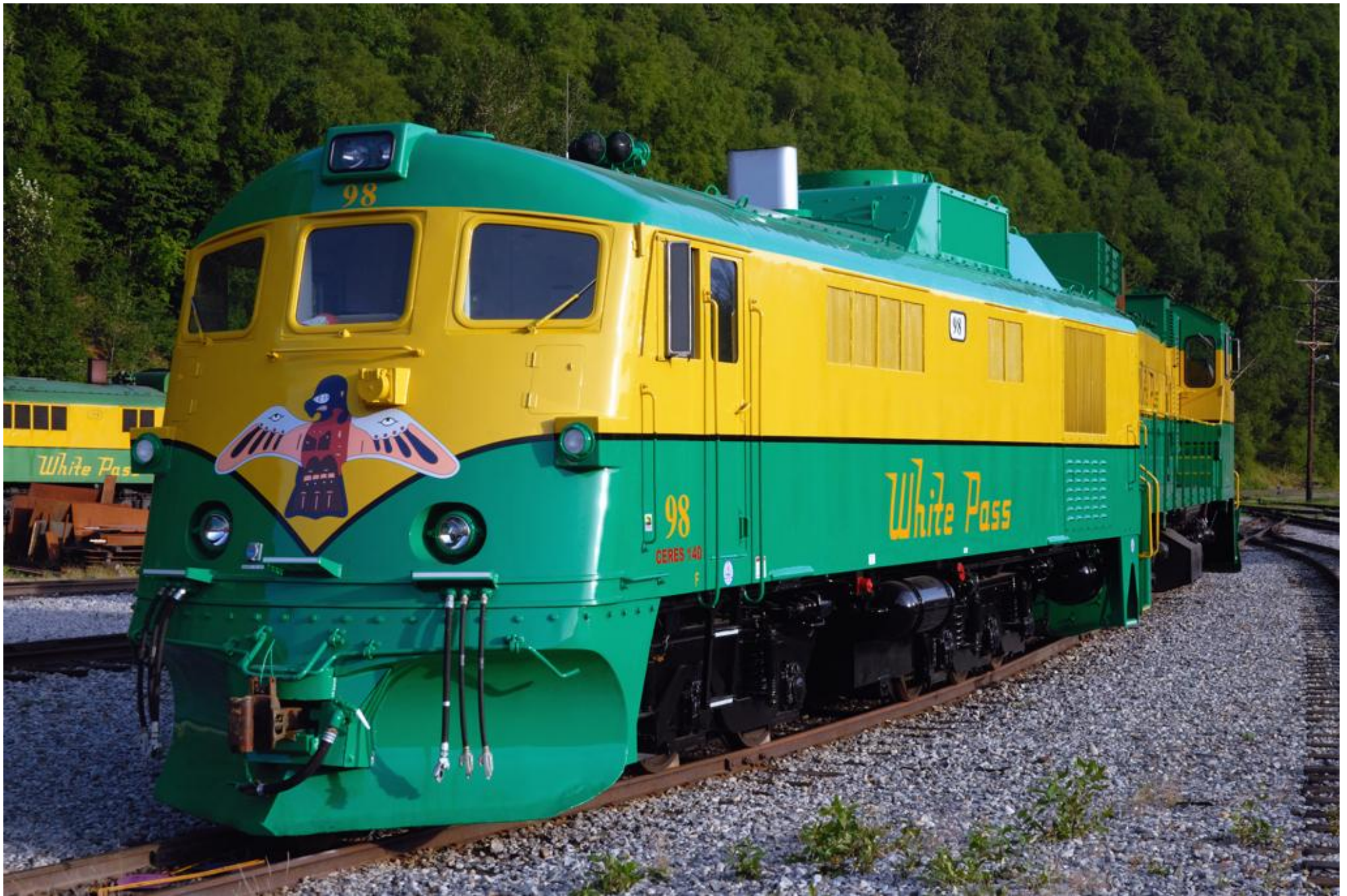
#98, having completed its initial setup at Skagway is ready to enter revenue service. Apparent in this photo is the placement of the dynamic brake to the area formerly occupied by the winterization hatch. Ditch lights with removable covers have been added along with an external roof mounted radiator. It is expected two CERES 140's will replace three conventional units. Skagway 7/13/09 Photo by Deane Motis
