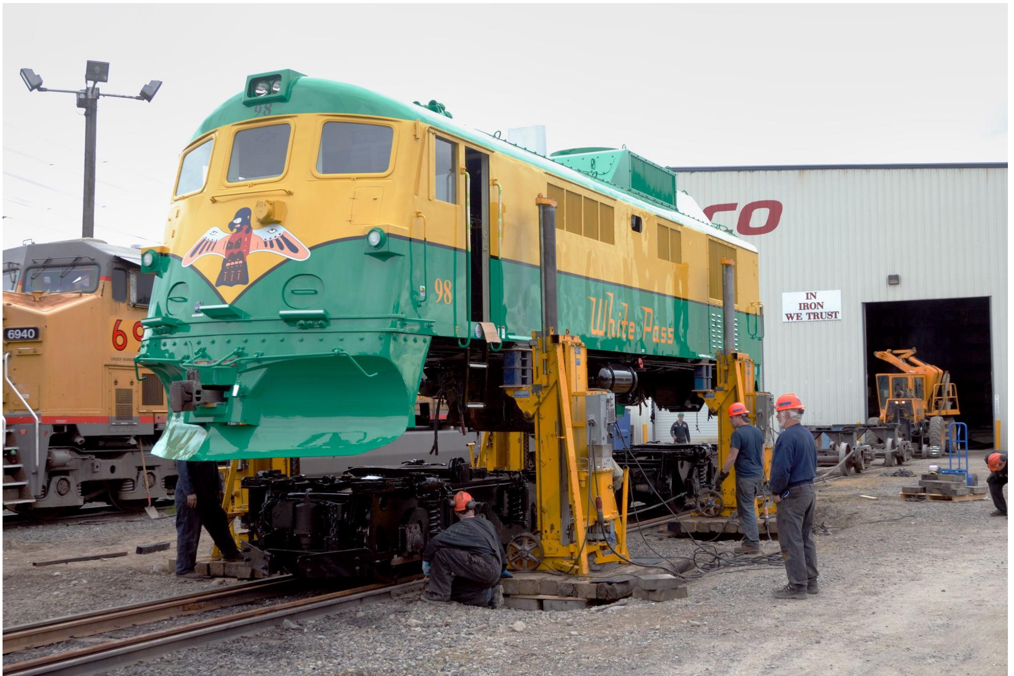
Having been rolled out in late May, 2009, 98 prepares to exchange its standard gauge shop trucks for its double equalized CC trucks. Four 35 tonne jacks were used to lift the unit 9 feet in the air in order for the trucks to clear the plow. Tacoma, WA 5/8/09 Photo by Deane Motis
